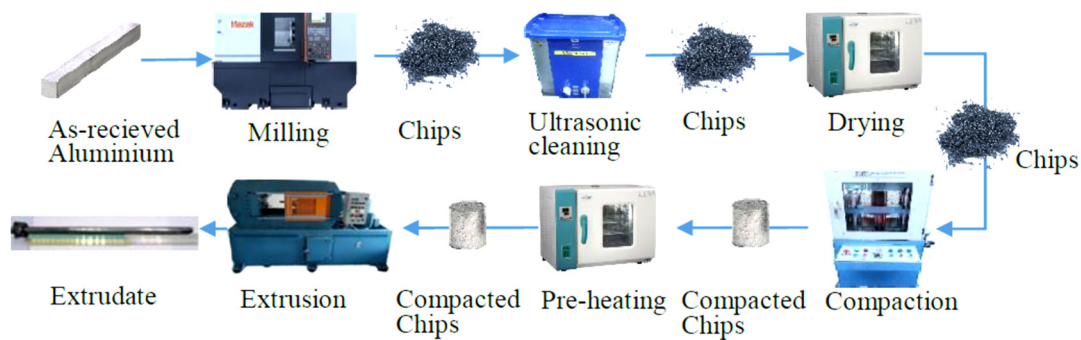
Figure 3. Extrusion procedure in recycling aluminium chips.
