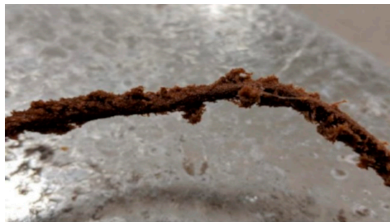
Figure 1. Poly( \epsilon -caprolactone (PCL)/ sawdust (SD) extruded wire with SD content of 50 wt.%.
