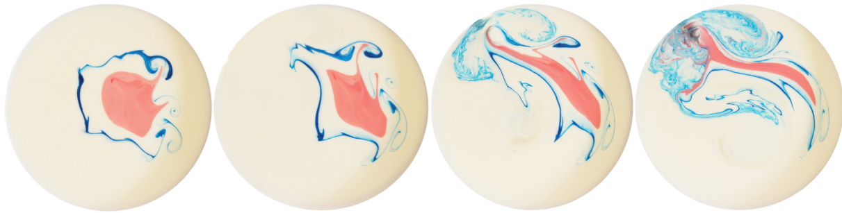
Figure 1. A photograph of the scalar mixing process: three fluids (white, red and blue) arranged on a plate (150 mm diameter) and stirred by a rotating disk (5 mm diameter, 7600 rpm). Pictures taken at about 5 s intervals (courtesy of Zofia Waclawczyk (2020)).
