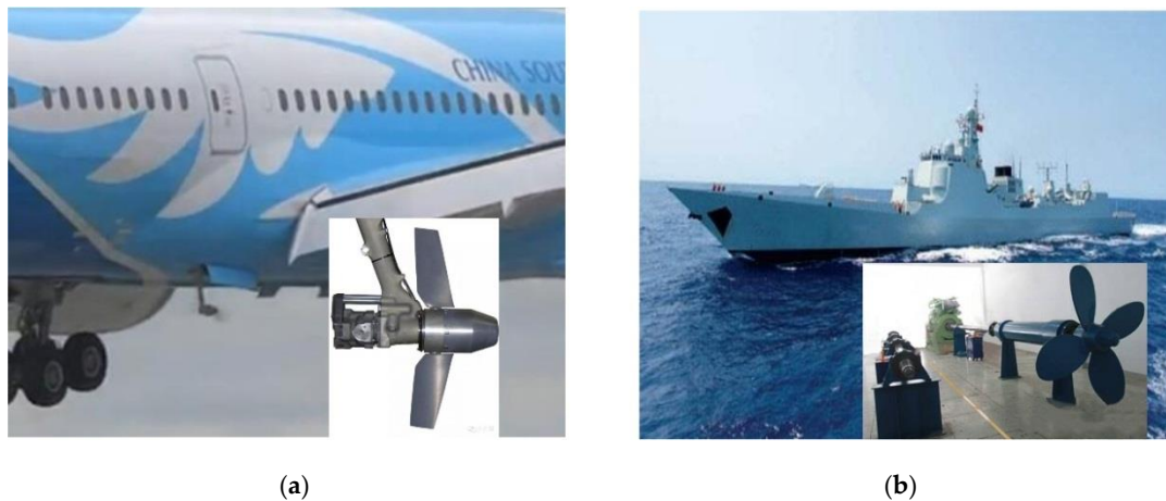
Figure 1. The industry application of gear coupling-rotor system (GCRS). (a) Application in the ram air turbine of aerospace. (b) Application in the propulsion shaft system.
