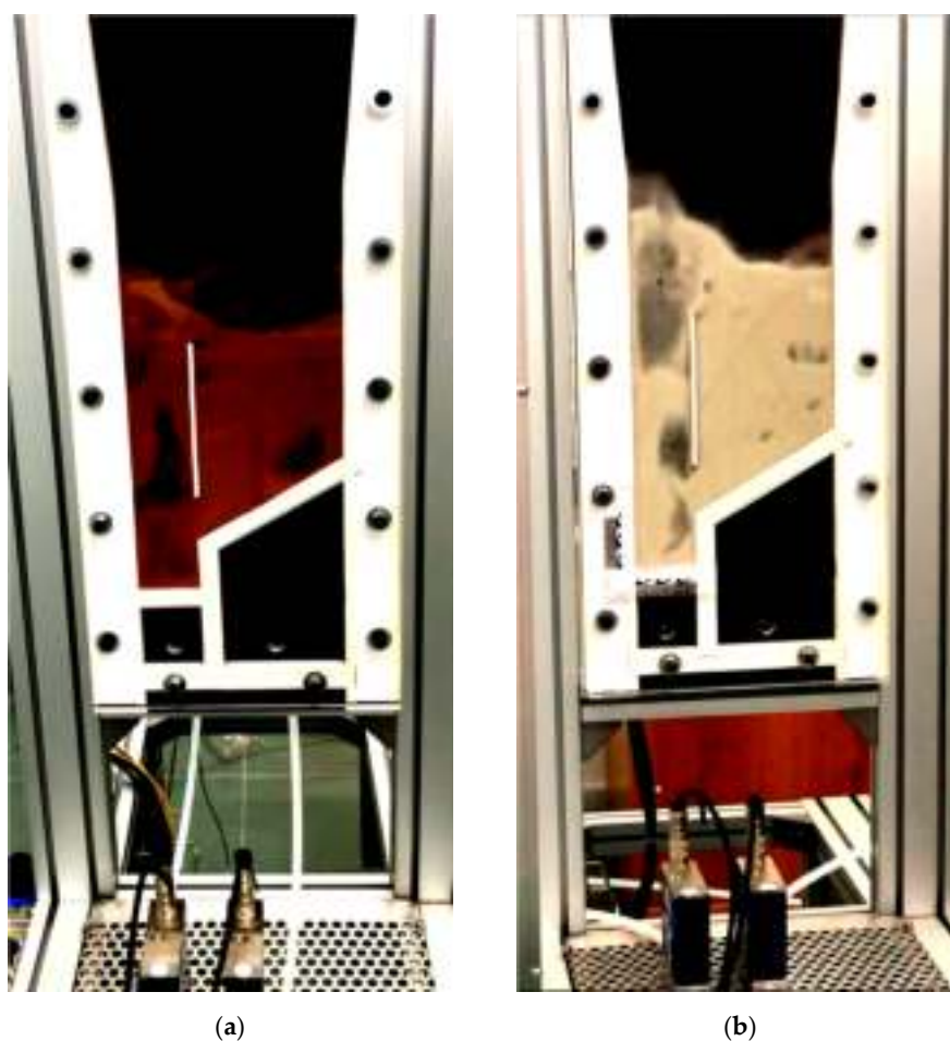
Figure 3. ENEA's ICBFB pseudo-2D cold model test ring implementing LaVision PIV system for velocity field evaluations. Images of test conducted with: (a) 0.14 mm copper powder particles; (b) 0.55 mm glass beads.
