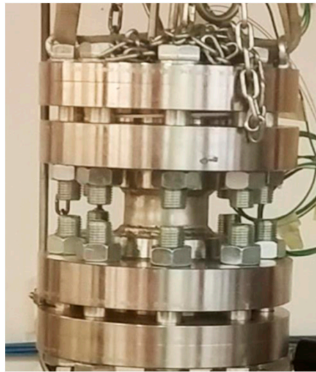
Figure 2. Image of the lab-scale apparatus used for hydrate formation tests.
