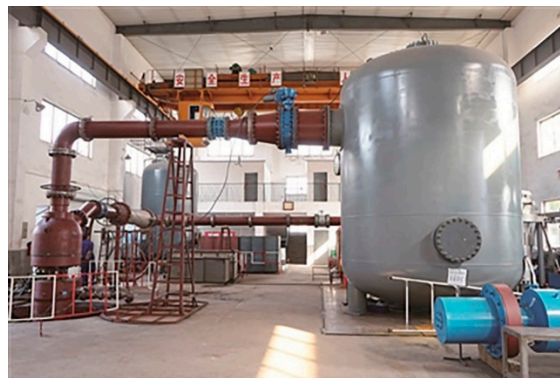
Figure 5. Test bench of boiler circulating pump.
