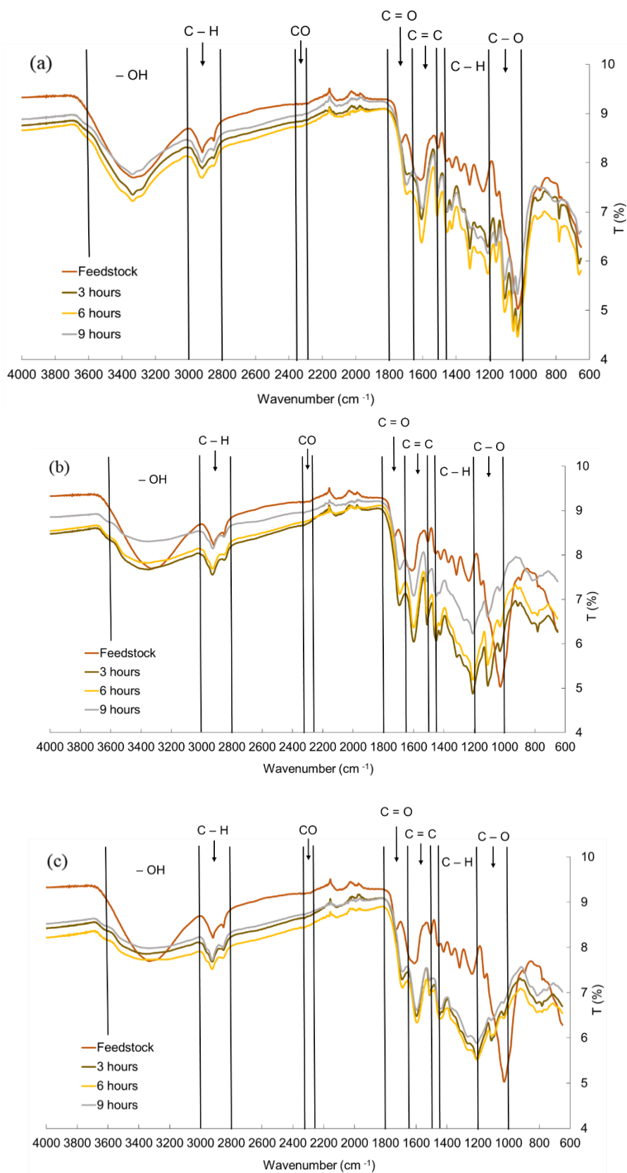
Figure 8. Fourier-transform infrared spectroscopy (FTIR) spectra depending on the reaction time for each reaction temperature. (a) 220 °C; (b) 250 °C; (c) 280 °C.
