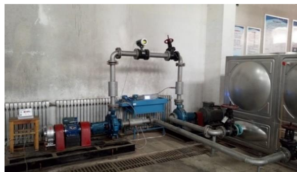
Figure 7. Experimental equipment of PAT. (a) Schematic diagram of experiment; (b) test rig.
