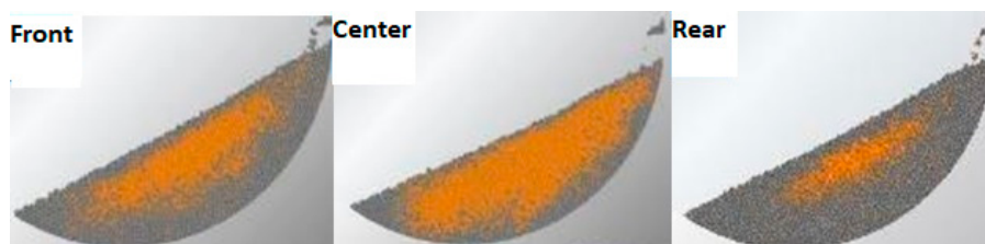
Figure 8. The simulated beads distributions after 2 min (6 revolutions) of mixing for the bi-size bed (drum filled at \frac{1}{4} , 4 baffles of 1.5 cm), from the left to right: front layer, center layer, rear layer.
