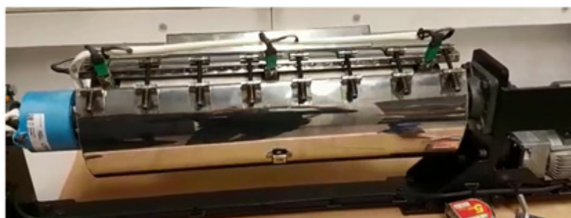
Figure 2. Torrefaction laboratory rotating batch reactor.
