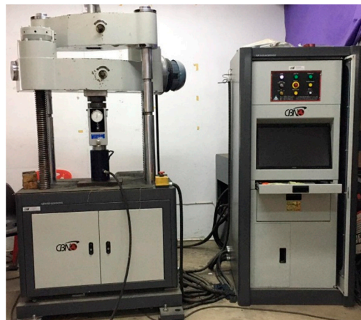
Figure 6. The tensile test machine (model CY-6040A1, c.b.n. testing corporation co. ltd, Bangkoknoi, Bangkok, Thailand).
