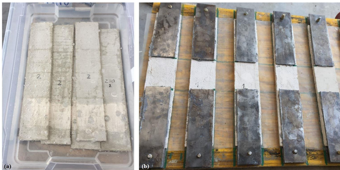
Figure 2. (a) Specimens immersed in saline solution and (b) the application of metal tabs on FRCM coupons.
