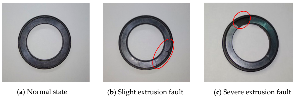
Figure 3. Rotating ring in different extrusion fault.
