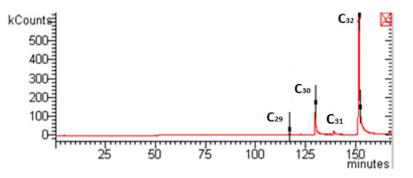
Figure 4. Example of a GC-MS trace related to waxes collected in the I separator at -14 °C and 100 bar.
