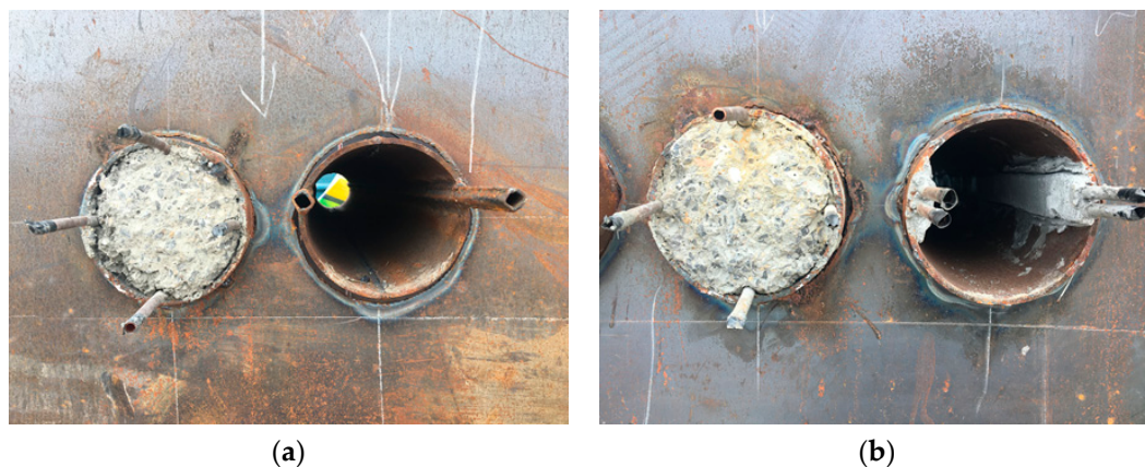
Figure 6. Exterior view of model. (a) Model showing profiled freezing-tube (Configuration 1). (b) Model showing double circular freezing-tubes (Configuration 2).
