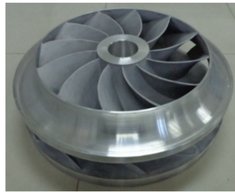
Figure 3. Experimental sample of centrifugal fan.
