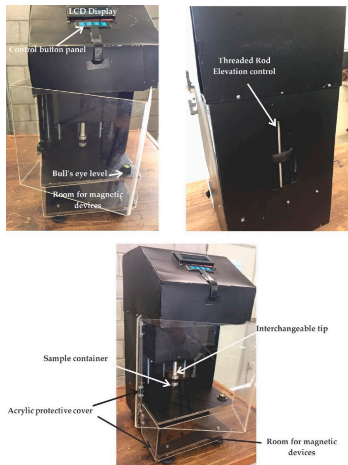
Figure 15. Manufactured rheometer—final version. Product specifications: power source 110V, sensor power source 12 V, variable speed operation from 0 to 1000 RPM, interchangeable test probes, ability to incorporate attachments to perform electro- and magneto-rheological tests.
