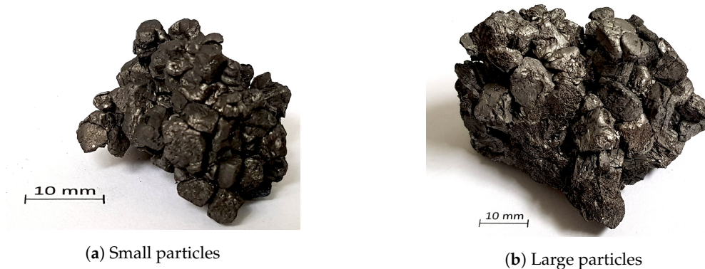
Figure A7. Images of coal char agglomerate from pyrolysis at 1600 °C using (a) small particles and (b) large particles.
