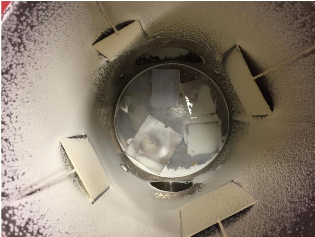
Figure 4. Current deposition pattern in unit 5 when running 8.8% milk powder at 170 °C.
