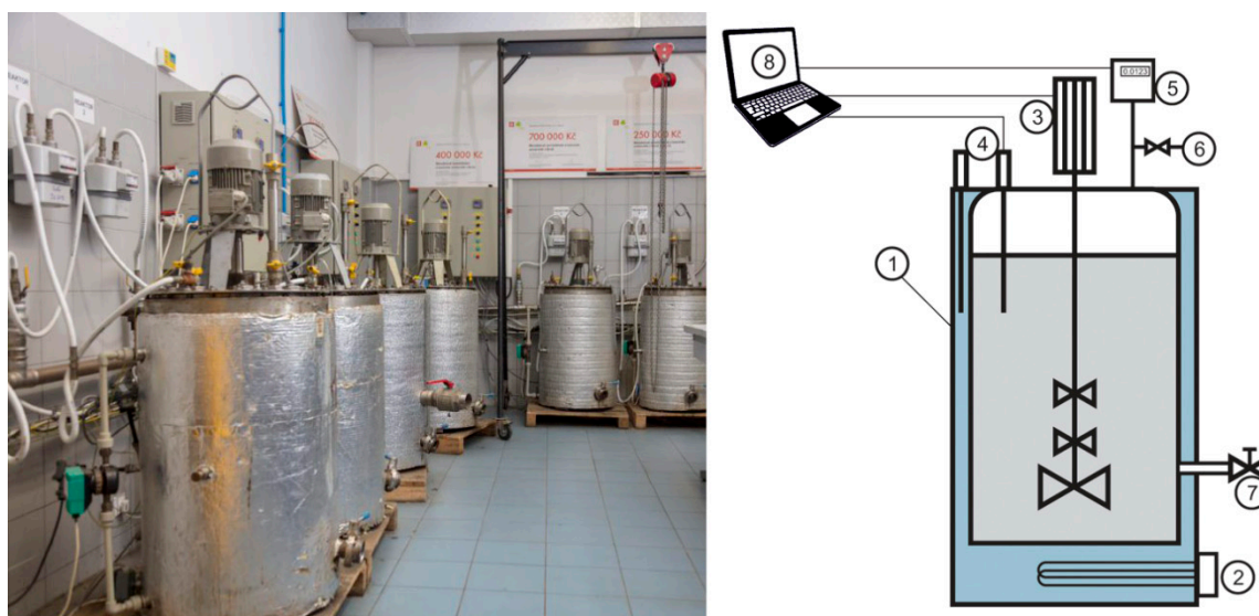
Figure 1. Lab view and fermenter scheme, (1) hot-water heating system, (2) electric heating coil, (3) electric-driven agitator with a frequency converter, (4) two temperature sensors for hot-water and fermenter content, (5) gas meter, (6) sampling point for biogas analysis, (7) sampling point for the fermented substrate and (8) computer control system.
