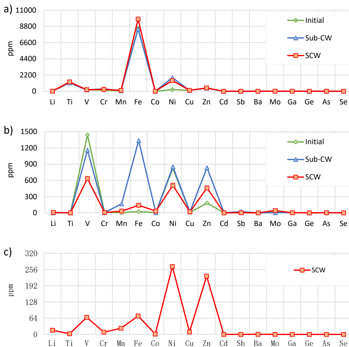
Figure 6. Distribution of trace elements in (a) rock samples, (b) asphaltenes, and (c) carbene-carboids of Domanic shales before and after sub-CW and SCW experiments.
