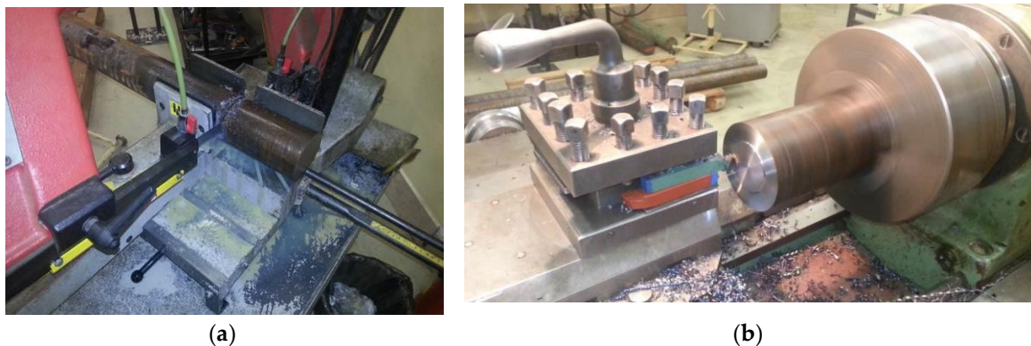
Figure 8. Carrying out of experiments – material cutting (a), face alignment (b).
