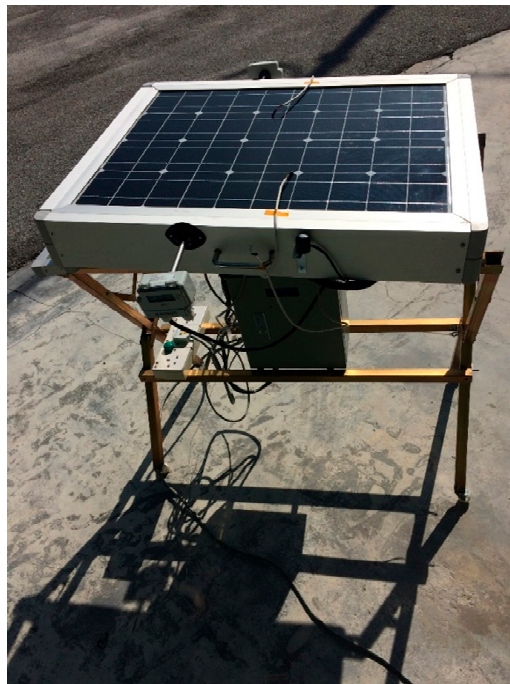
Figure 5. Experiment set-up for data collection of the PV/T solar collector.
