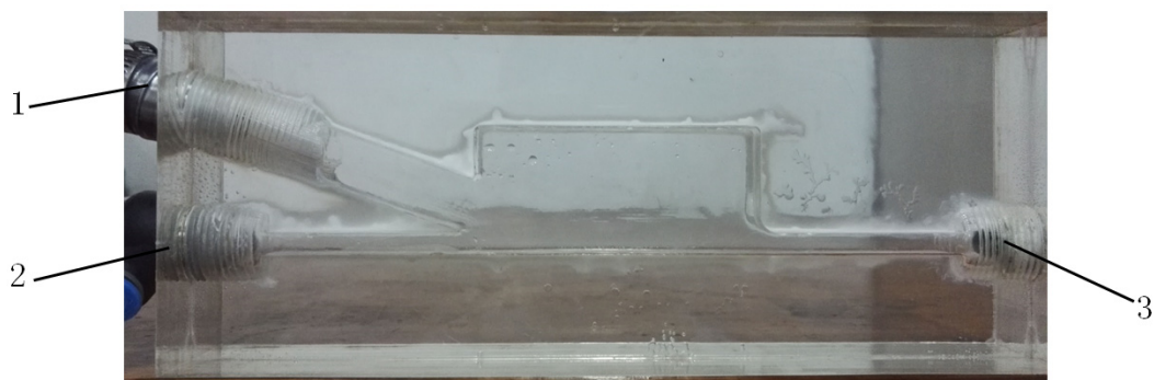
Figure 16. PIV observation flow channel: 1. particle flow inlet, 2. micro-nano-bubble inlet, 3. outlet.
