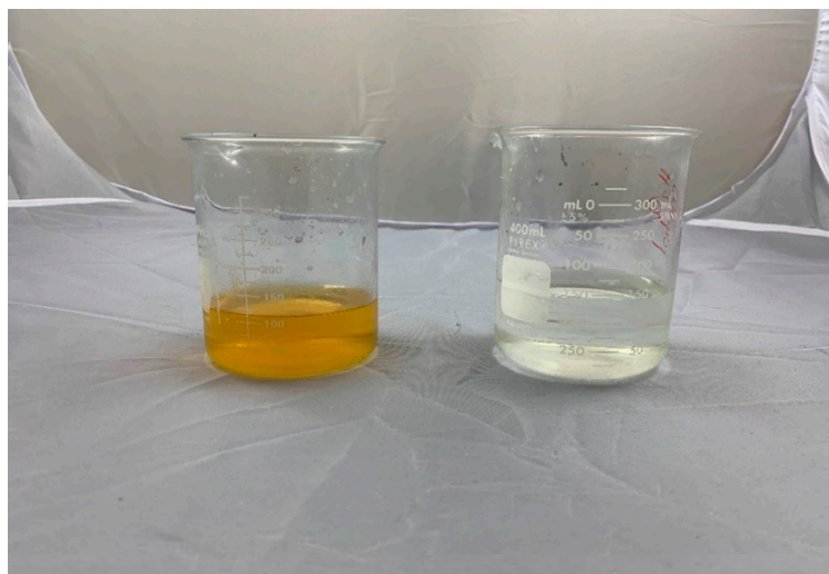
Figure 8. Comparison of water released following filtration after treatments with poly(PLA 4 ChMA) (left) and poly(TMAEMC) (right).
