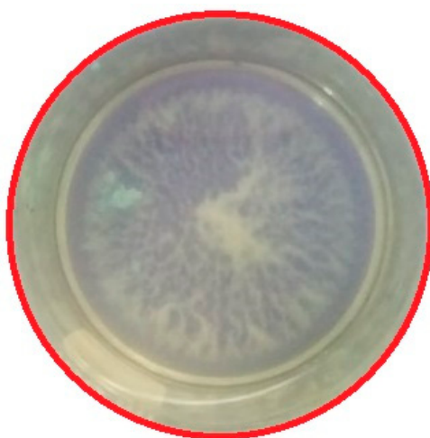
Figure 9. Photographic view of the solid residue produced during plasma treatment of industrial wastewater.
