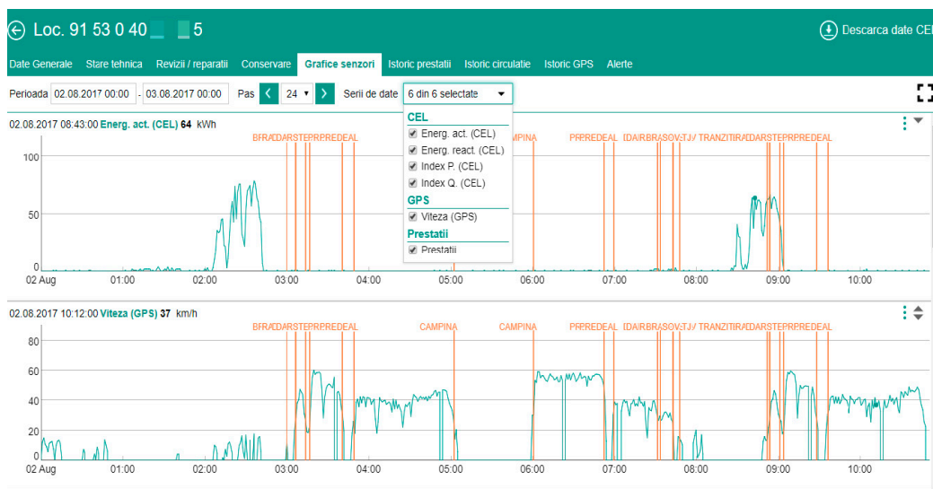
Figure 5. Display in the web-server application of train information, with correlated information for a train, information for DL1 and DL2/DL3, train speed, fuel or electricity consumption, and geographical identification (screen captures). Observation: the user interface of the application is in Romanian but we aim to improve this aspect in the future stage of application development.
