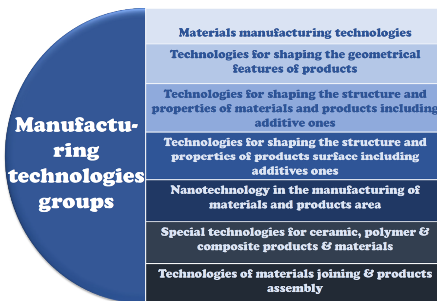
Figure 9. General classification scheme of product manufacturing technology.
