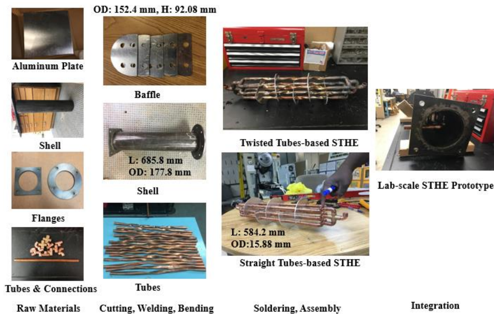
Figure 3. Fabrication process of the lab-scale STHE prototype.
