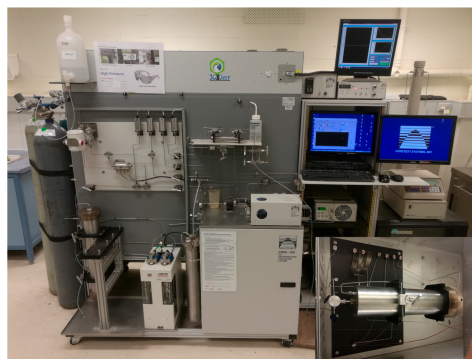
Figure 2. Core flooding set-up for permeability tests.
