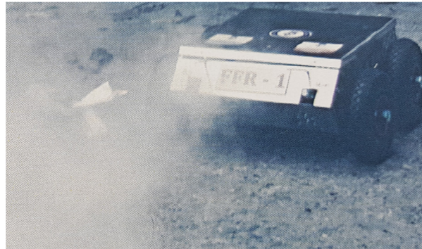
Figure 6. Unmanned ground vehicle (UGV) performing fire extinguishing testing, carried out at the Military Technical Academy yard on 26 October 2017, at the Patriot Fest contest.
