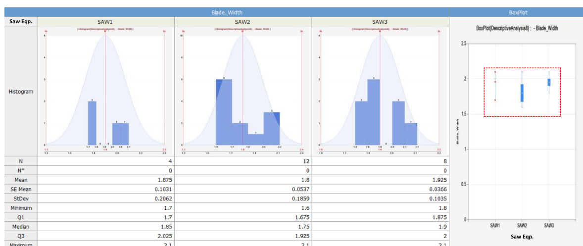
Figure 7. Analysis of difference in the blade widths among the wafer sawing process equipment.
