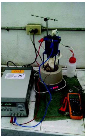
Figure 1. Bench-scale fixed bed adsorber prototype.
