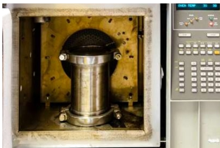
Figure 2. One liter tank in oven (Hewlett Packard 5890 GC) ready for heating.
