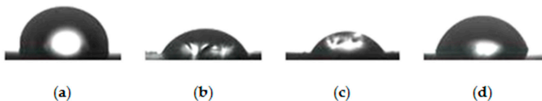
Figure 7. Image wetting test for the contact angle at 8 min for sample (a) JPU, (b) JPU/GO 0.35 wt%, (c) JPU/GO 0.50 wt%, and (d) JPU/GO 0.65 wt%.
