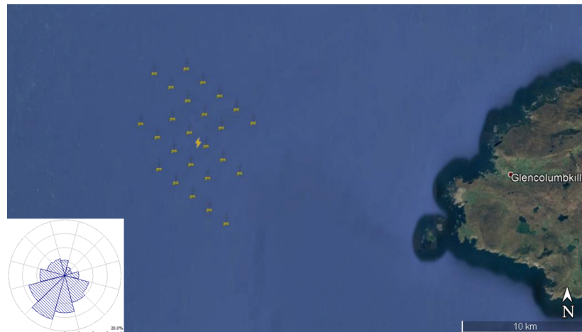
Figure 10. Farm arrangement, position of the offshore substation (bolt symbol), and wind rose of the site, showing the wind frequency per sector.
