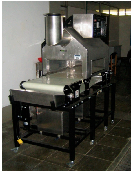
Figure 2. Refractance window equipment for drying guava slices.
