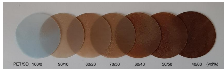
Figure 1. Effect of wood content (0–60 vol.%) on recycled-PET wood plastic composite (rPET WPC) color. SD = sawdust.
