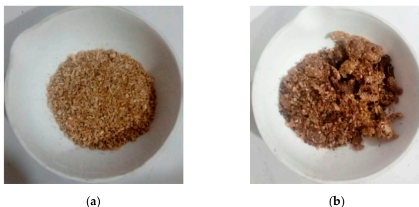
Figure 5. Fragments of biomass particles in melting PP with feed containing 0% weight of PP (a), combined flocks and fragments of biomass particles in melting PP from a sample taken when co-pyrolysis with feed containing 25% weight of PP (b). Samples were taken when co-pyrolysis achieved 300°C.
