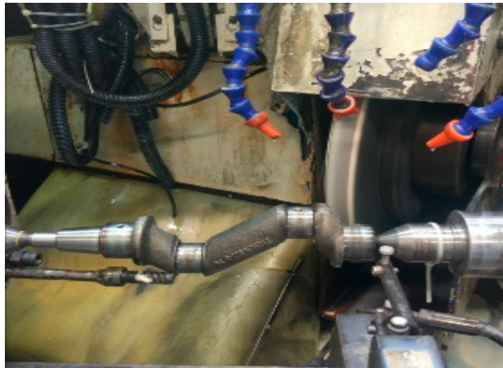
Figure 5. Actual machining of the crankshaft.
