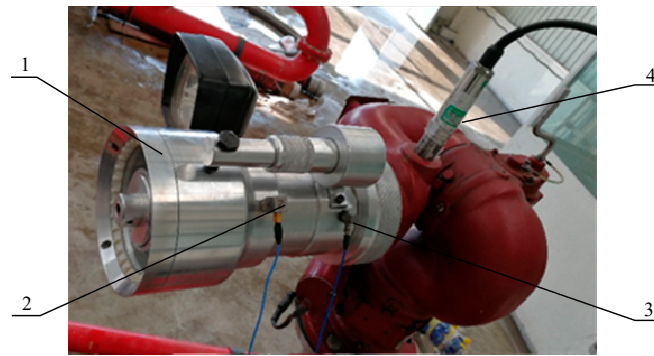
Figure 18. The fire-fighting monitor prototype and sensors. The labels are as follows: 1. Fire-fighting monitor 2. Acceleration sensor (three directions), 3. Acceleration sensor (one direction), and 4. Pressure sensor.
