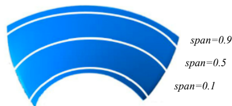
Figure 9. Impeller blades with different radial coefficients.
