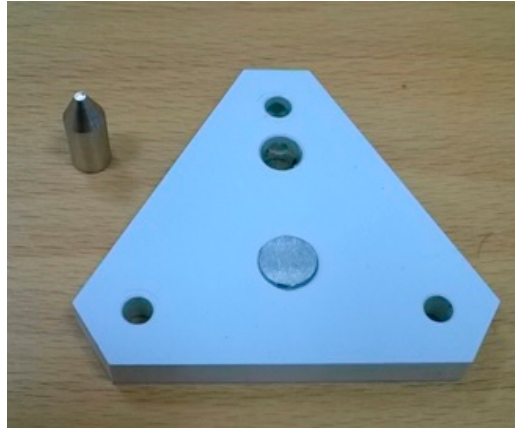
Figure 3. Sample mounted in a holder and a counter-sample used for the tests.
