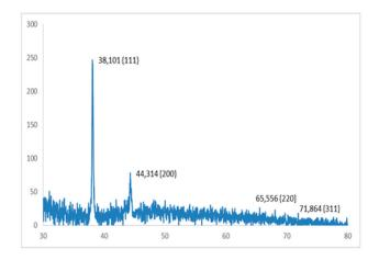
**Figure 8.** XRD pattern of triangular silver nanoplates stabilized by the mixture of gelatin 0.2 (%, w/v) and chitosan 0.06 (%, w/v) at pH 6.0.
