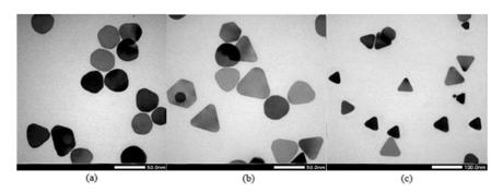
**Figure 4.** TEM images of (a) nano disk shapes (scale 50 nm) (G + CHI 0%, w/v); (b) hexagonal (30%) and triangular shapes (50%) (scale 50 nm) (G + CHI 0.5 + 0.06%, w/v); and (c) high yield of triangular shapes of AgNPs (70%) (scale 100 nm) (G + CHI 0.2 + 0.06%).
