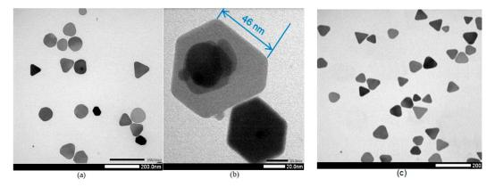
**Figure 2.** TEM images of (a) the nanodisk shapes (scale 200 nm) (75  $\mu$ L AgNO<sub>3</sub> 0.01 M); (b) the hexagonal shapes (scale 20 nm) (125  $\mu$ L AgNO<sub>3</sub> 0.01 M); and (c) high yield of triangular shapes (80%) of silver nanoplates (200  $\mu$ L AgNO<sub>3</sub> 0.01 M) (scale 200 nm).
