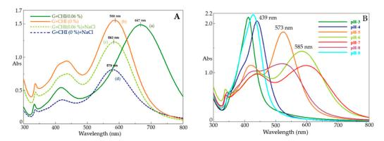
**Figure 5.** (**A**) UV-Vis spectra of triangular AgNPs colloidal dispersions synthesized with chitosan 0.06% (w/v) (gelatin 0.2%, w/v) (curve a), without chitosan (gelatin 0.2%, w/v) (curve b), with the presence of chitosan 0.06% after adding NaCl 1.0 M (curve c), and without chitosan after adding NaCl 1.0 M (curve d). (**B**) UV-Vis spectra of triangular AgNPs synthesized at different pH values (from 3.0 to 9.0) with gelatin (0.2%, w/v)-chitosan (0.06%, w/v).
