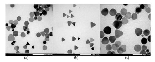
**Figure 6.** TEM images of silver nanoparticles synthesized mixed gelatin (0.2%, w/v)-chitosan (0.06%, w/v) solution at (**a**) pH 4.0, (**b**) pH 6.0, and (**c**) pH 8.0 (scale 100 nm).
