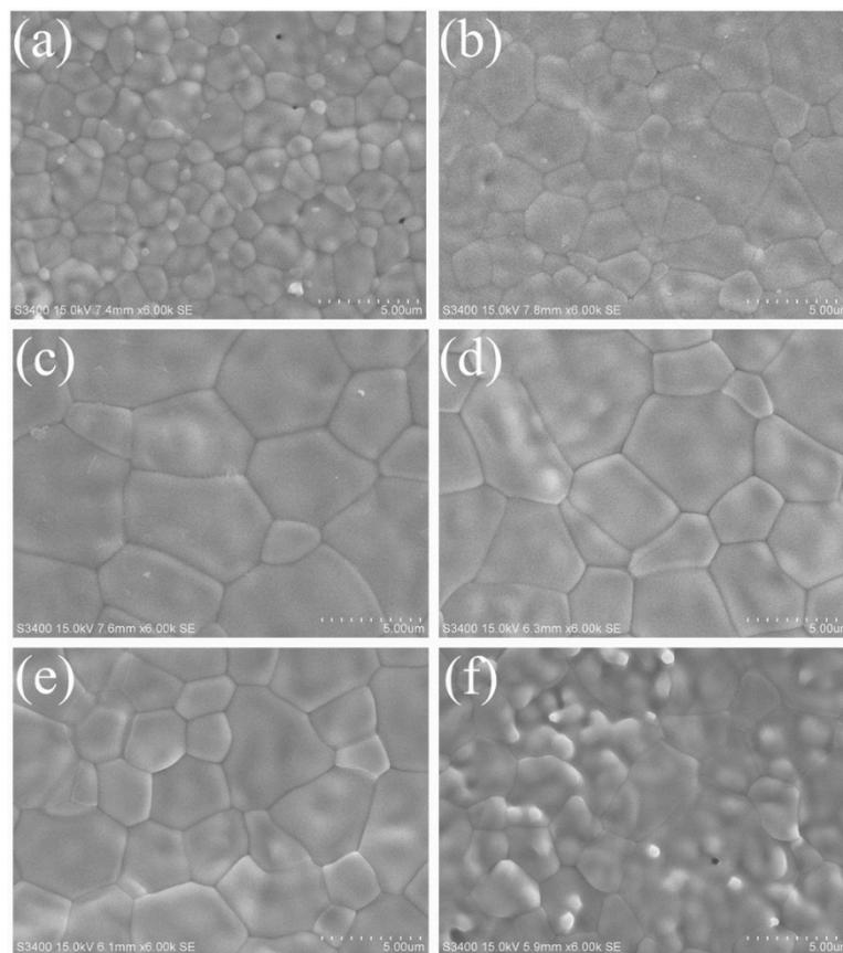
**Figure 3.** SEM images of sintered SCGZ with 0.5 wt% CuO at (a) 1423 K, (b) 1473 K, (c) 1523 K, (d) 1573 K, (e) 1623 K and (f) 1673 K.
