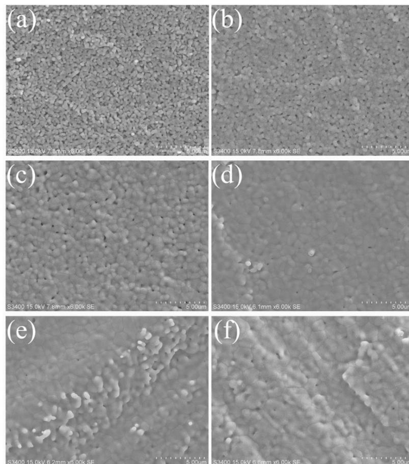
**Figure 2.** Scanning electron microscope (SEM) images of sintered  $\text{Sc}_{0.1}\text{Ce}_{0.05}\text{Gd}_{0.05}\text{Zr}_{0.89}\text{O}_2$  (SCGZ) at (a) 1423 K, (b) 1473 K, (c) 1523 K, (d) 1573 K, (e) 1623 K, and (f) 1673 K.
