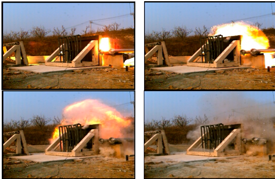
Figure 11. Structural response of rear-face-strengthened wall specimen in test 3.
