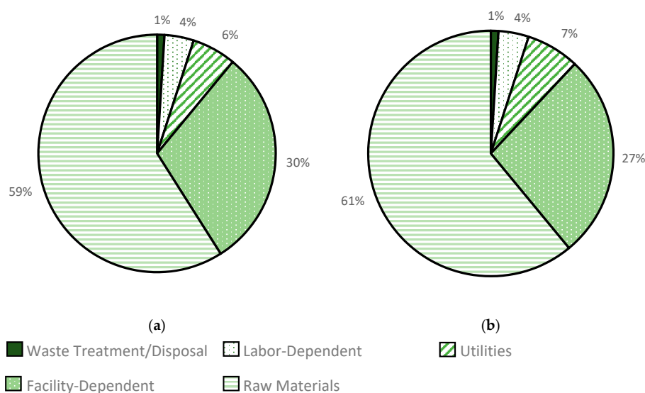
Figure 2. Annual operating cost breakdown for (a) batch SuperPro Designer base case and (b) fed-batch SuperPro Designer base case.
