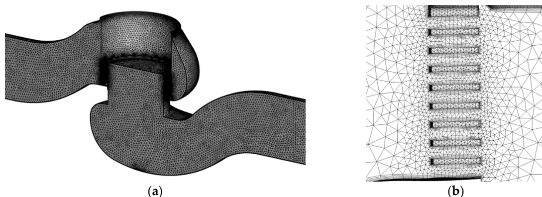
Figure 2. Mesh of the sleeve regulating valve with maximum valve core displacement of 60 mm (a) overall view; (b) mesh in the sleeve.
