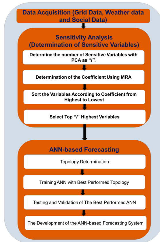
Figure 2. Proposed methodology for the Artificial Neural Network (ANN) based-forecasting system.
